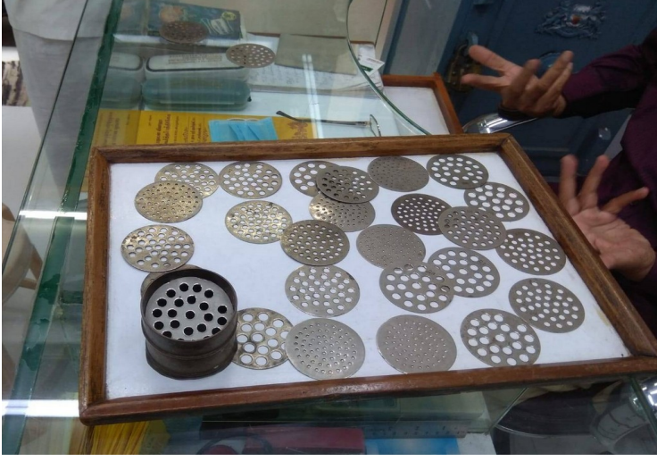
Image 1: Pearl Sieves, for Sorting and Grading of Pearls. Image courtesy Muthu V. Prakash
